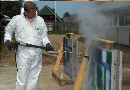
The participants were asked to evaluate and judge the results based on result, cost, speed and environmental impact and among the 4 different ways of attacking the problem (2 chemical product ranges, sodablasting and lavablasting) the lavablasting won with a narrow margin to the use of a chemical product range used by Luke Murphy of INTELblast Spain.
